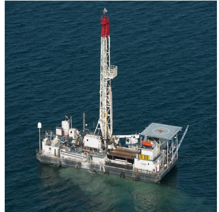
Dundee drilling barge
